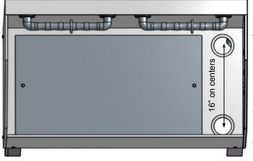
Center of each drain hole is 5" from inside of front/back wall
