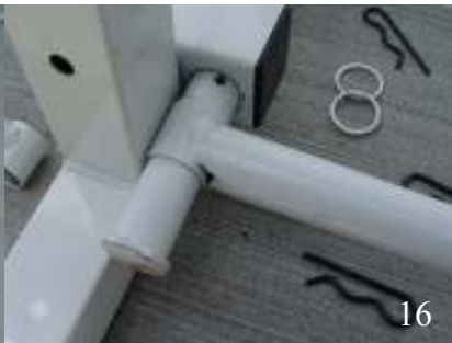
16. There are 4 pairs of part #4s. They are of telescopes type in the same size. Connect outer rod ends to the bottom of the bases, and connect inner rod ends to the back of center board #2 and ramp #1, #3. Remove the cotter pins and washer rings and connect #4 to the base #8 one by one.
