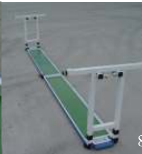
8. Connected part #8 to part #2. They should look like it shown in picture 8. Then, flip them back to up right position shown in picture 9. Make sure to adjust each base #8 straight up as a right angle to board #2.
