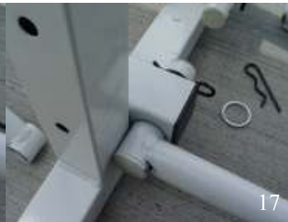
17. Correct connection should look like shown in picture 17. There is a twisting knob on each telescoping rod #4 to let them slide or tighten up. Loosen the knob first before pulling out the inner rod to connect the other ends to the back of board and ramps.
