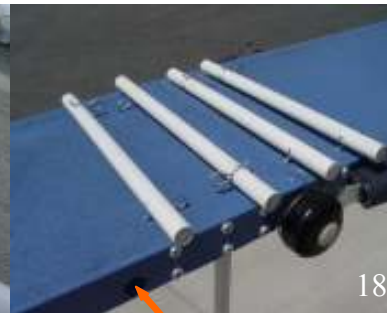
18. There are 4 #11 parts, the rods for connect part #4 to back of the board and ramps. There are 2 pair of holes on the side of center board and one on each side of ramps. (see the arrow) Remove cotter pins and connect #4 inner rod ends to back of the board and ramps.
